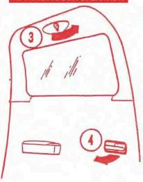
To open aft cabin door, twist upper door latch (3) forward. Pull lower door latch (4) out. Push door open.
