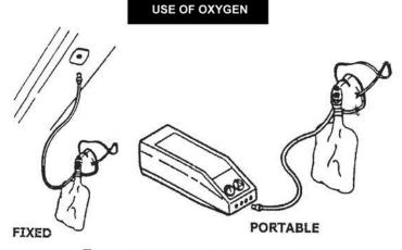
To use oxygen, insert fitting into receptacle. (twist to lock) and don mask.
