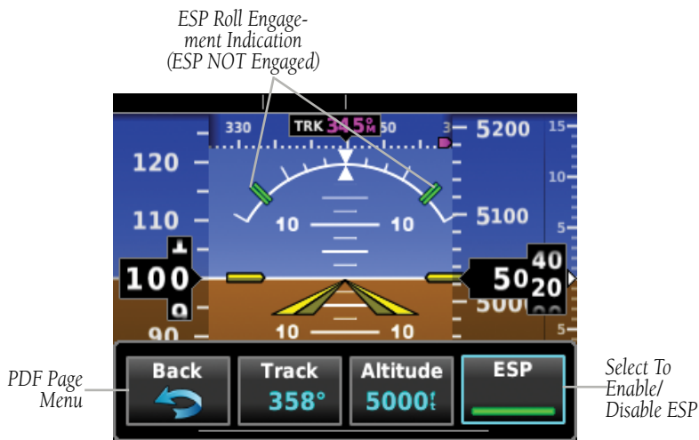
Figure 3-25 AFCS (ESP Enabled)
