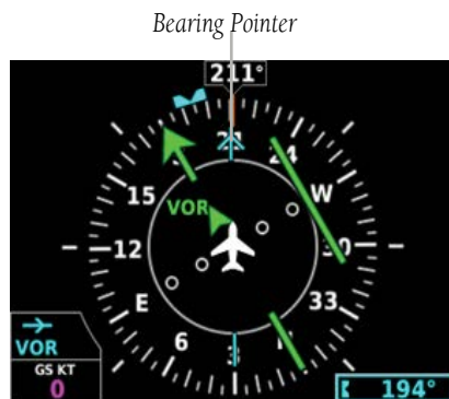
Figure 2-17 VOR Source Bearing Pointer
