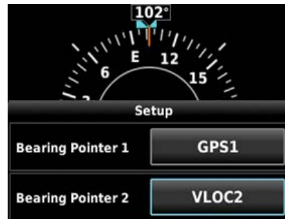
Figure 2-19 Bearing Pointer Setting
