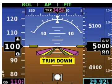
Figure 3-22 TRIM DOWN Alert
