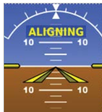
Figure 1-4 Attitude Aligning Indication
