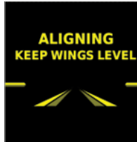
Figure 1-5 Attitude Aligned Keep Wings Level Indication
