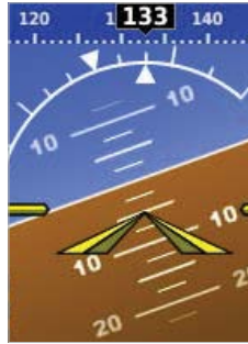
Figure 2-7 Ground Pointer Configuration
