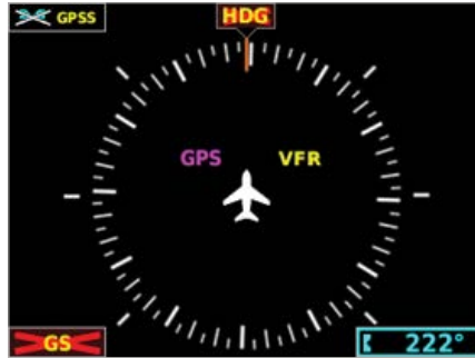
Figure 1-3 G5 HSI Page Failure Annunciations
