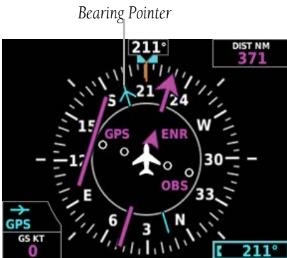
Figure 2-16 GPS Source Bearing Pointer
