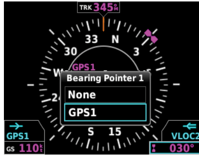
Figure 2-20 Bearing Pointer Source Options
