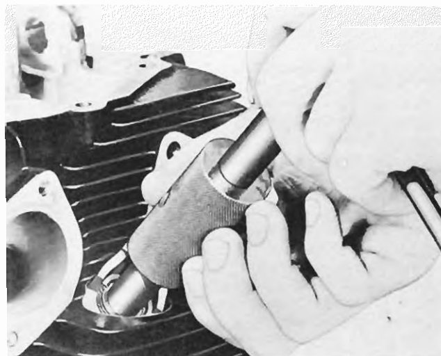
Figure 106 - Installing Heli-Coil Insert
