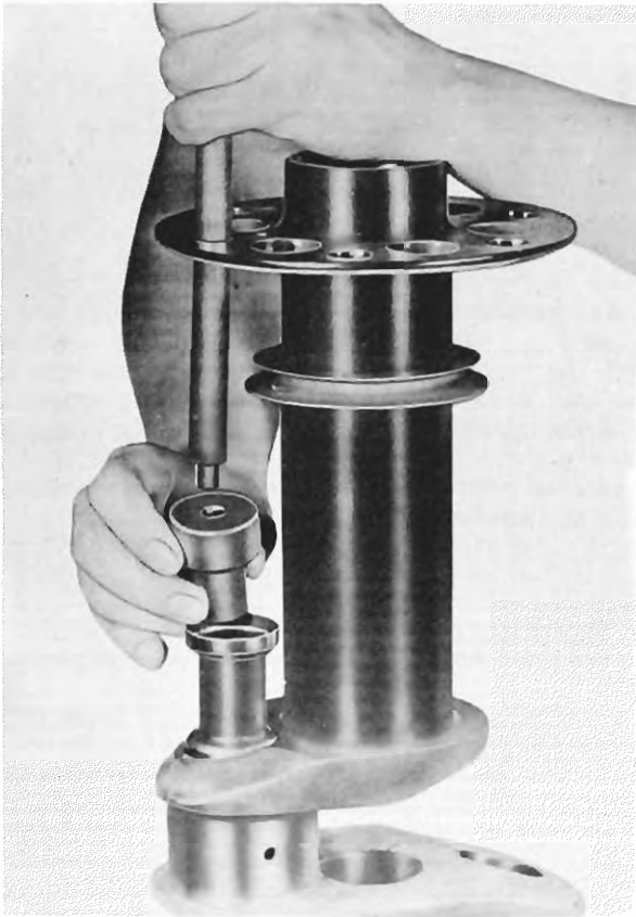
Figure 120 - Installing Crankpin Oil Tubes
