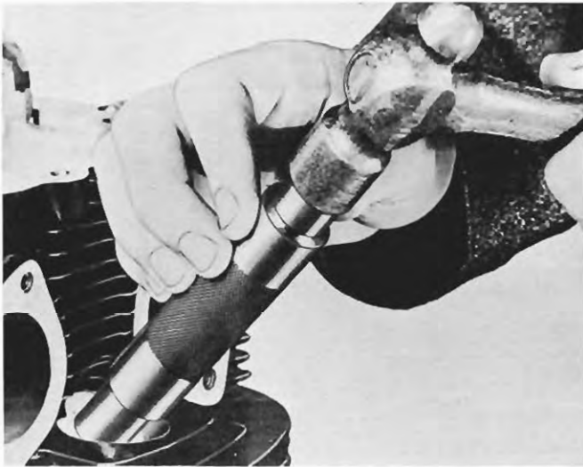
Figure 108 - Staking Heli-Coil Insert
